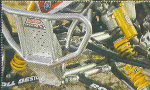
■ ABOVE The IMS-Roll GP Series Nerf Bar and Heel Guard provide excellent protection, as well as stability.
