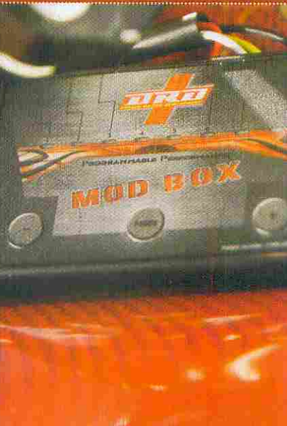
■ BOTTOM RIGHT The DRD Mod Box is preprogrammed by Dubach himself to supply your Raptor 700 with just the right amount of fuel for his exhaust system.
