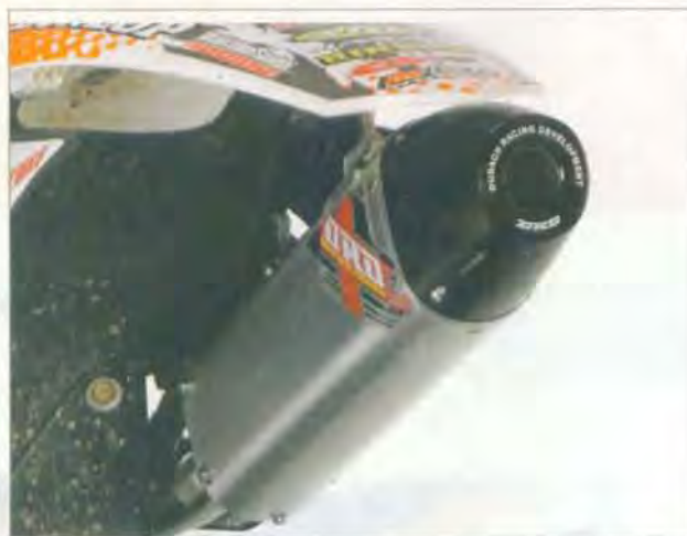
The new rear can is 2 1/2 inches longer than a normal DR.D can. It also has a smaller end cap, special core and quieter cough than the standard motor design.
