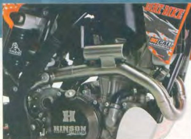
The PHD header was originally brainstormed nearly 100 years earlier. The concept of absorbing and releasing exhaust pressure targets improved bottom power. DR.D fit a Hinson inner hub and clutch cover for durability and looks.
