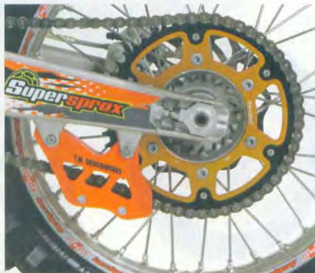
The Supersprox sprocket proved incredibly durable, as did the TM Designworks chainguide. Both are excellent off-road mods.
