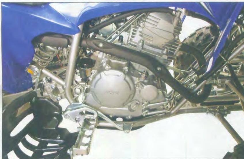
*In stock form, the 250R makes about 15 horsepower. That's not much, but handling and light weight are the traits that make the machine a hit. Most riders only complain about the lack of reverse.*
