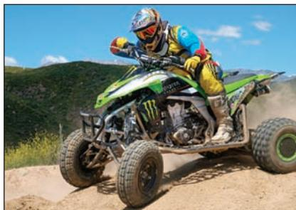
**With only KX450 cams, a Fuel Customs airbox, a DR.D pipe & a Mod Box, the KFX was the fastest machine in the mod squad.**
