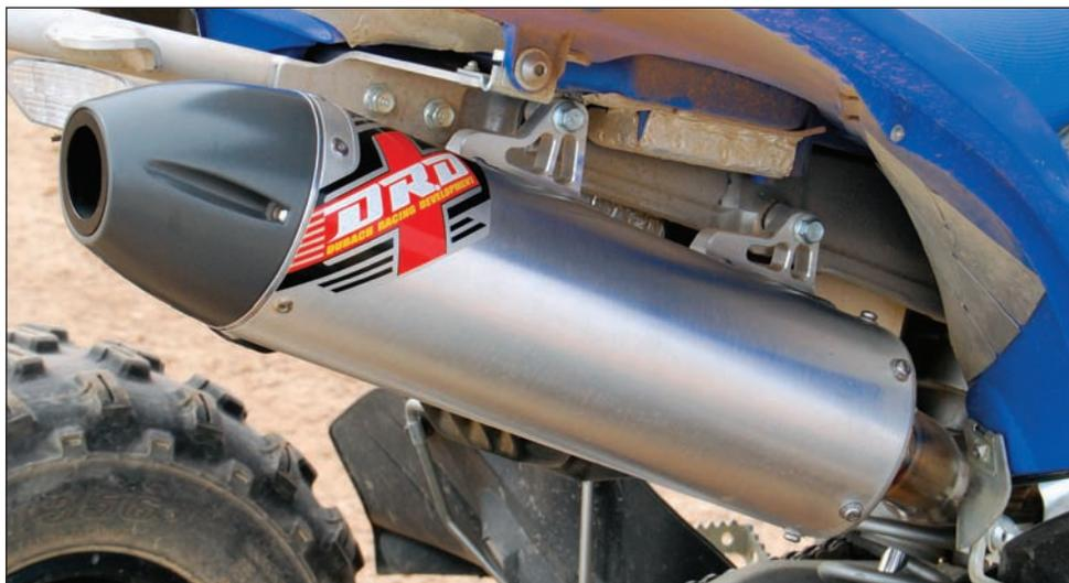
*The muffler can is aluminum, with an aluminum endcap and spark arrestor insert as well. DR.D includes a special wrench to disassemble the muffler when it's time to repack it. Sound levels ring about 97.8 dB on our sound meter, which isn't too obnoxious.*
