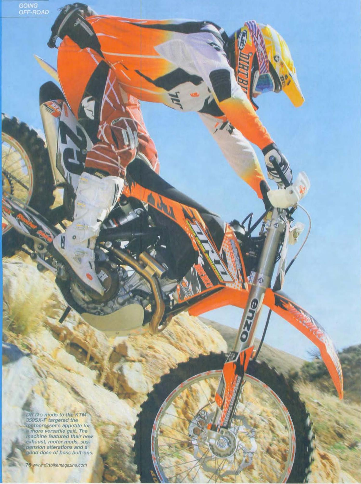
*DR.D's mods to the KTM 350SX-F targeted the motocrosser's appetite for a more versatile gait. The machine featured their new exhaust, motor mods, suspension alterations and a good dose of boss bolt-ons.*
