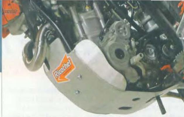
Ricochet's skid plate is thick, takes hits quite well, but does need some foam under the frame rails to quiet it down.
