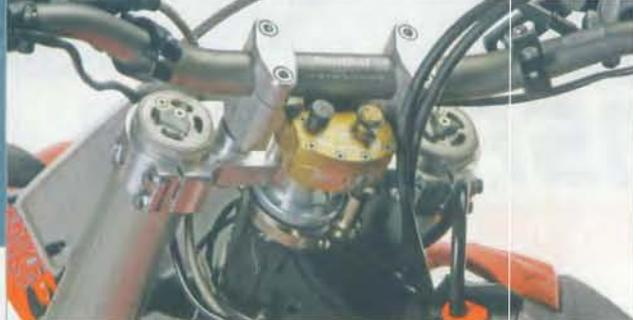
Rubber-mounted Applied 18s improve the front tire's contact patch and offers quicker manners. The Scott's damper helps to ward off any front-end sneezing that may have arrived courtesy of the faster traits.
